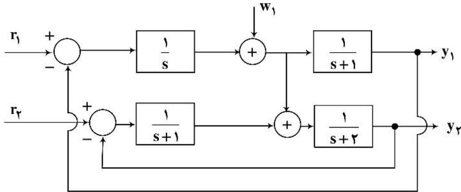
$$\frac{Y_2(s)}{R_1(s)} = \frac{(s+1)^2}{s(s+1)^2(s+2) + s(s+1) + (s+1)(s+2) + 1} \quad (1)$$
